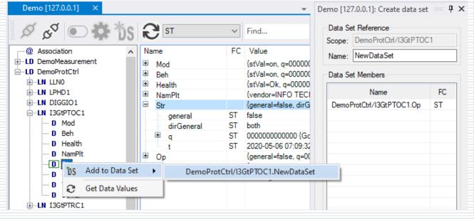
When the list of elements is complete, press **Create** button – a command will be sent to the server device.
