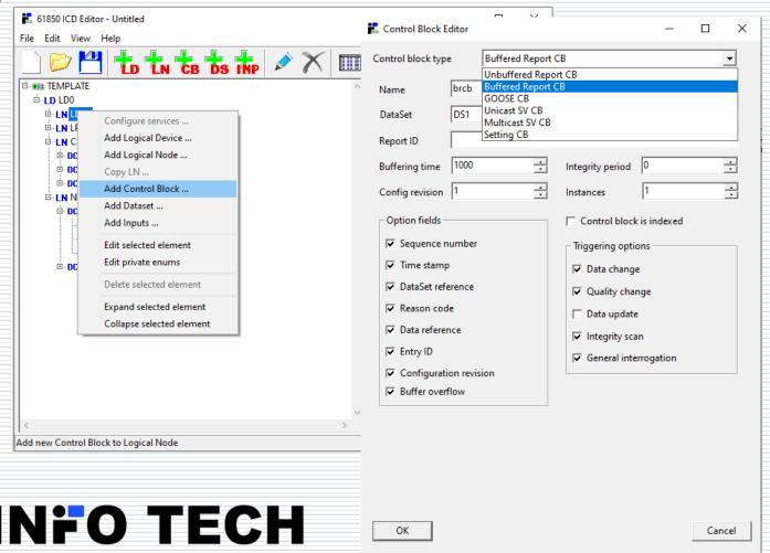
URCB, BRCB, GoCB, USVCB, MSVCB and SGCB can be added to the data model and initially preset.
