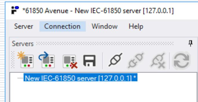
\* **after** the name of the IED server device means **unsaved configuration**.
