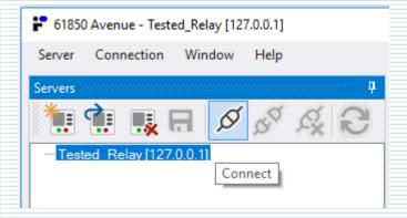
Now the client-server connection can be established: in **Server** window from context menu of the selected device invoke the command **Connect**
