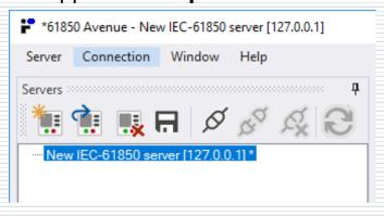
\* after the name of the IED server device means unsaved configuration.
