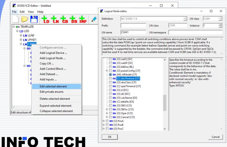
Any added LN can be later modified by adding/deleting optional DOs and DAs.
