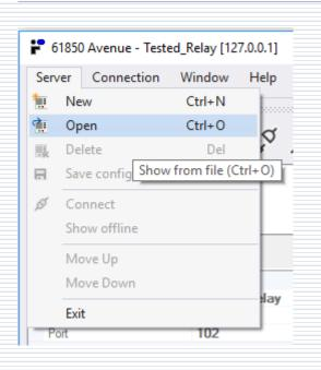
Invoke **Open** command and select an SCL file describing the server device.
