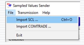
The sampled signals waveforms can be configured using a recording from an imported COMTRADE.
