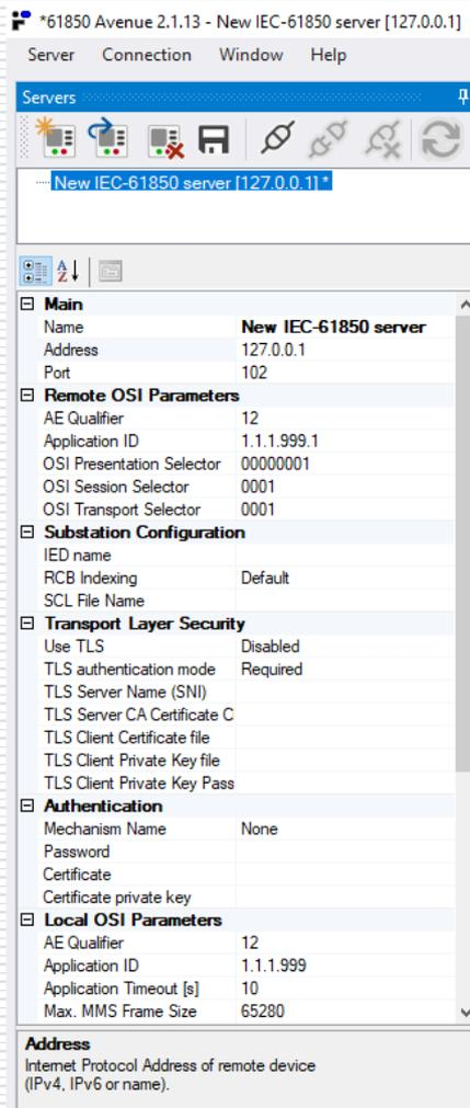
A new server IED with the name **New IEC-61850 server** and IP address **[127.0.0.1]** will appear in **Properties** window.
