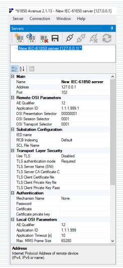
A new server IED with the name **New IEC-61850 server** and IP address [127.0.0.1] will appear in **Properties** window.
